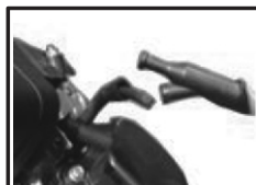
Pic.8 take off the ignition coil
